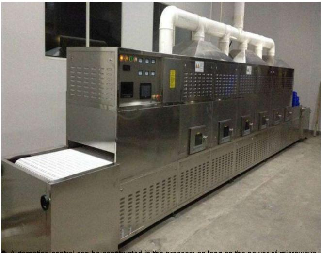
Automation control can be constructed in the process: as long as the power of microwave ripening sterilization equipment is controlled, instant heating and stopping can be realized without thermal inertia. The programmable control automation control of heating process and standard specification of heating process can be realized by using man-machine interface and PLC.
