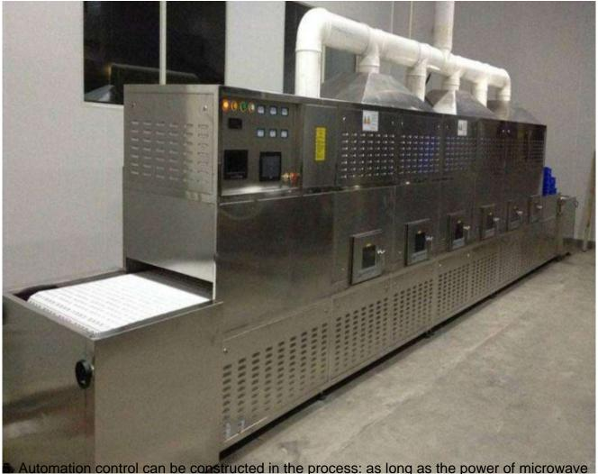
ripening sterilization equipment is controlled, instant heating and stopping can be realized without thermal inertia. The programmable control automation control of heating process and standard specification of heating process can be realized by using man-machine interface and PLC.
